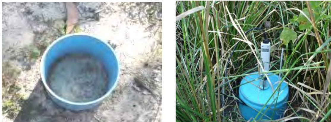
Figure 5 Gas chamber for sample collection (left) and measurement of CO 2 emission rate by portable CO 2 meter (right)
